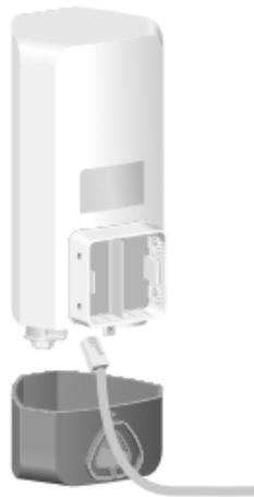
Figure 1-6 Connect Cables
